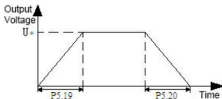
Fig. F5-7 Voltage Control Mode 2
