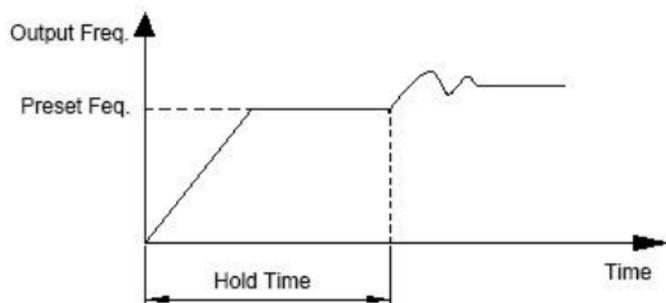
Fig. F8-4 Closed Loop Preset Frequency
