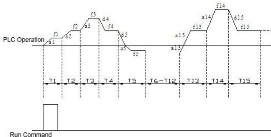
Fig.F9-2 Maintain Last Stage after Single Cycle
