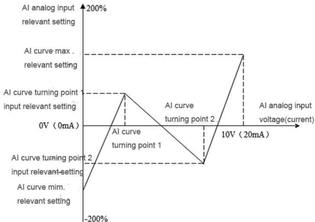
Figure F6-2 AI multi point curve diagram
