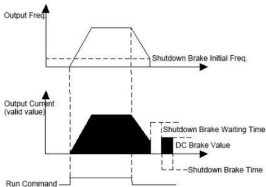
Fig. F1-4 Stop DC Braking
