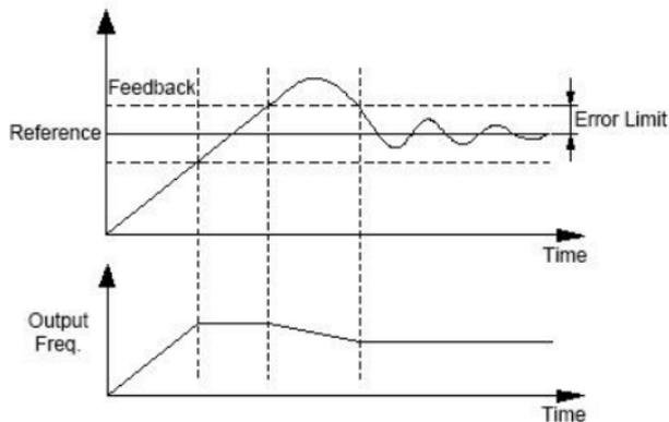
Fig. F8-3 Error Limit Schematic Diagram
