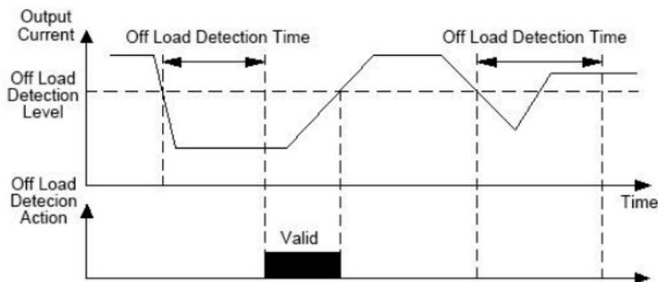
Fig. FA-3 Off Load Detection
