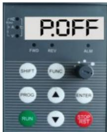
Fig 3-1 Power-on Parameter Display Initialization Display "P.OFF"
