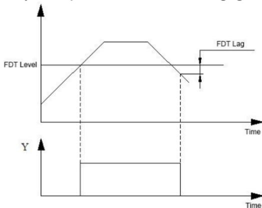
Fig.F7-8 Frequency Level Detecting
