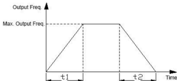
Figure F0-2 Accelerating and Decelerating time
