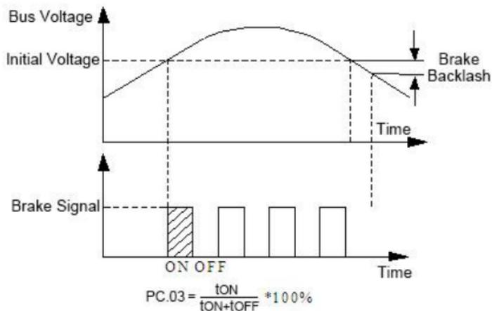
Fig. FC-1 Dynamic Braking
