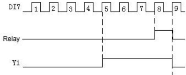
Fig. F7-9 Counter Reset and Detection Setting
