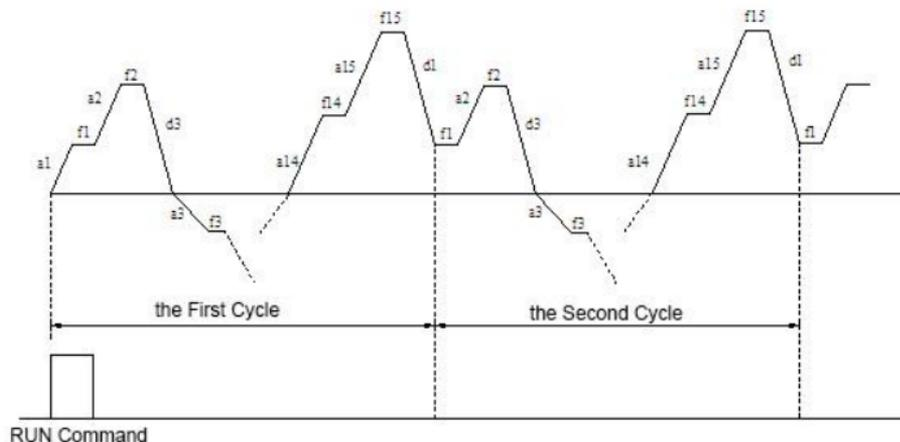
Fig.F9-3 PLC Continuous Cycle
