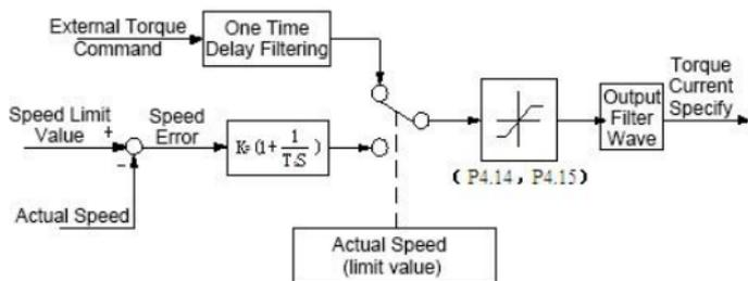
Figure F4-2 Torque Control Simplified diagram
