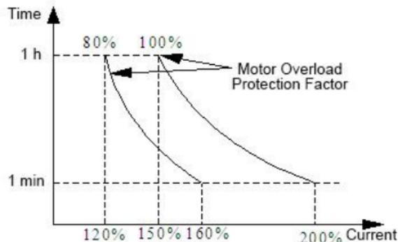
Fig. FA-2 Motor Overload Protection Factor Setting
