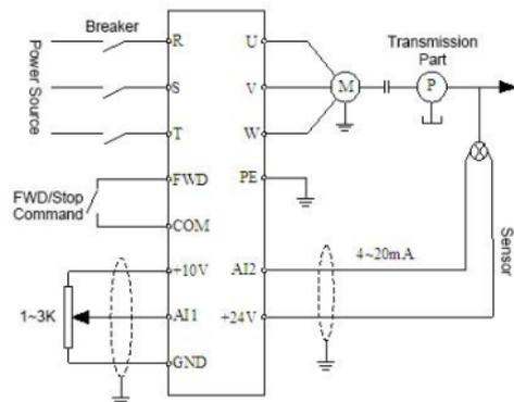
Fig. F8-1 Analog Feedback Control System
