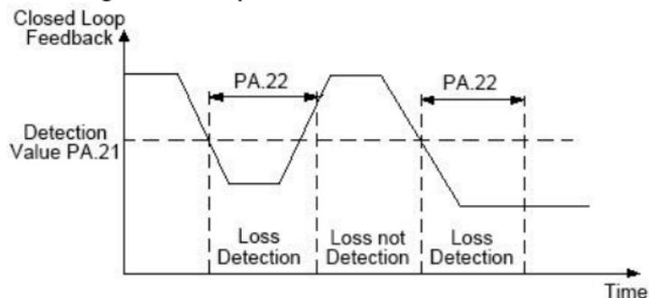
Fig. FA-4 Closed Loop Feedback Loss Detection
