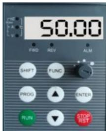
Fig 3-2 Stop Status Parameter Display Set Frequency "50.00"
