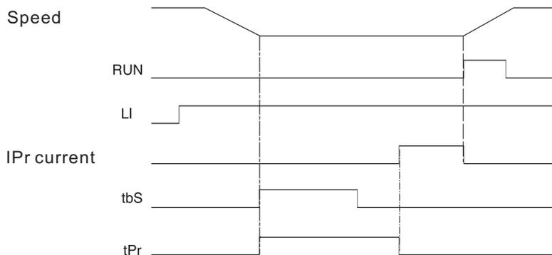
Preheating starts when the input is activated and the motor has stopped, after time delays tPr and tbS (PrO menu) have elapsed. Preheating stops if the input is deactivated, if a run command is sent or if the STOP input is activated.
